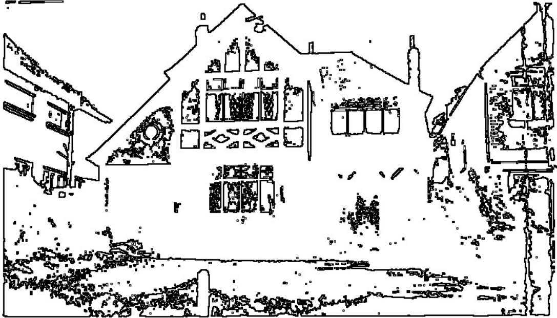
This is the output of a conventional edge detection algorithm on the binary image.
