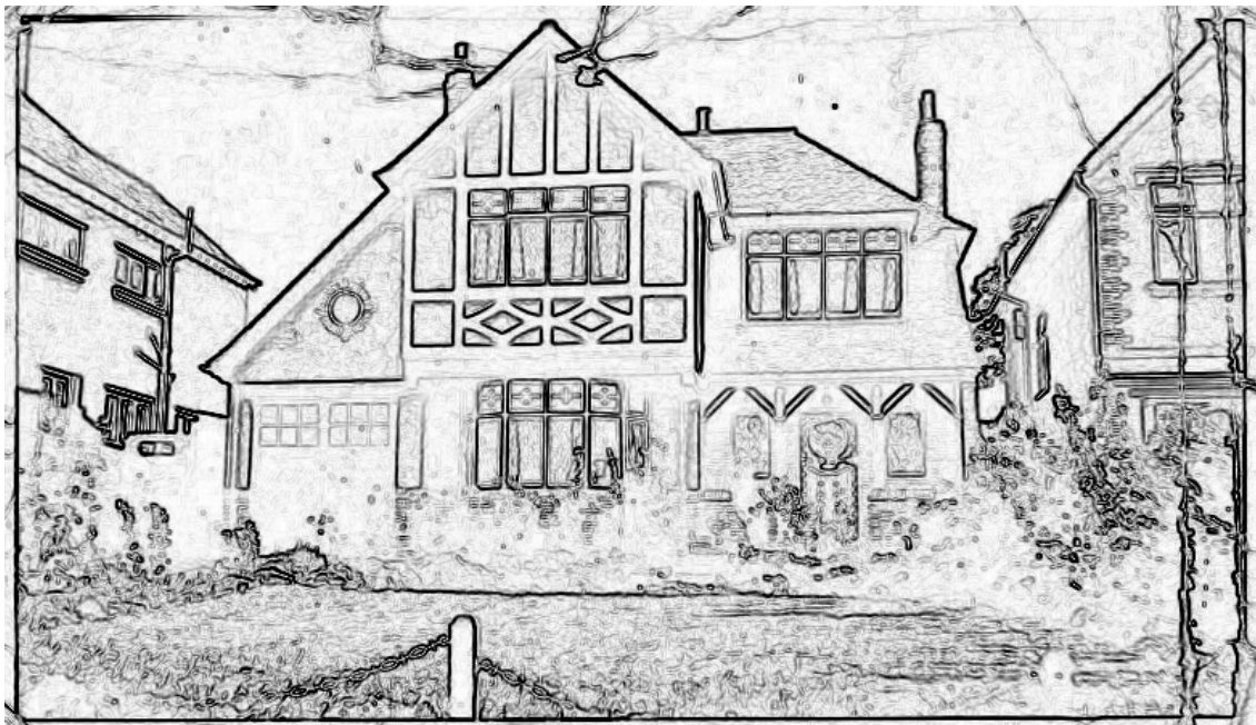
This is the output of a conventional edge detection algorithm on the 256 level greyscale image.
